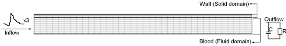
Figure 3: FEM of the aorta showing also the Boundary conditions for the fluid domain
